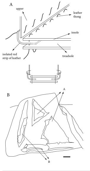
Figure 16. BM EA 4408/4409. A) The sole/upper construction. Not to scale; B) Openwork decoration of the instep flap. The letters are explained in the text. Scale bar is 10 mm. Drawings by E. Endenburg/A.J. Veldmeijer.
