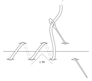
Figure 18. Whip stitching can be easily done from the outside by stitching at roughly right angle to the orientation of the previous stitch. Not to scale. Drawing by E. Endenburg/A.J. Veldmeijer.
